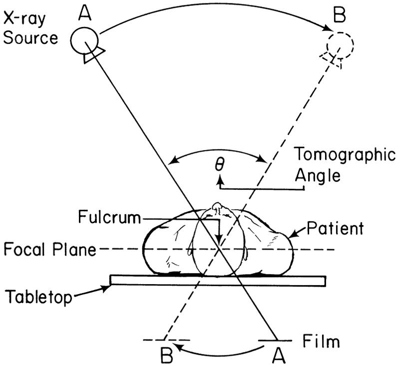
FIGURE 1. An example of a tomographic system.
