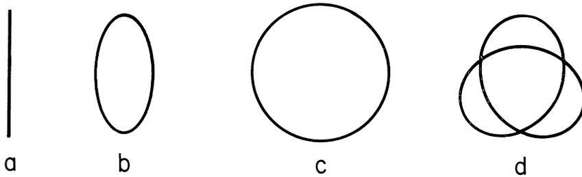
FIGURE 2. Tube-film motions used in tomography: a) linear, b) elliptical, c) circular, and d) hypocycloidal.
