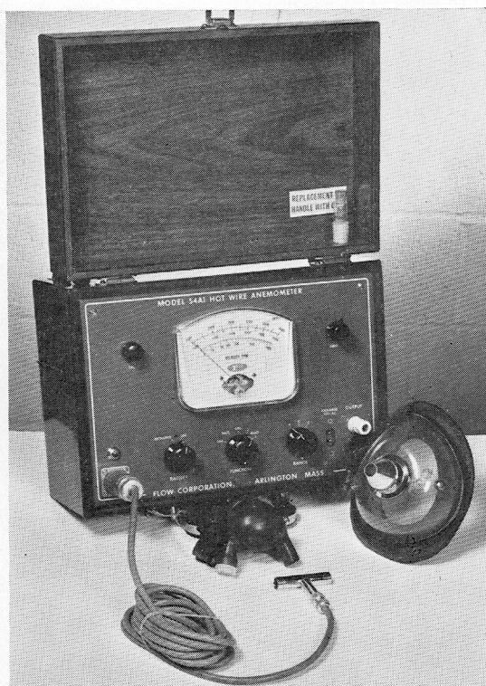
FIGURE 5. Warm wire anemometer with special T attachment for nasal, oral, or face mask.
