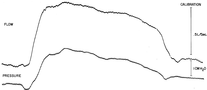
FIGURE 2. Pressure and airflow patterns from which nasal resistance was calculated. Pressure was measured at .5L/sec airflow.
