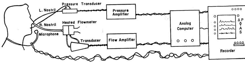
FIGURE 1. Diagrammatic representation of the analog computer system.
