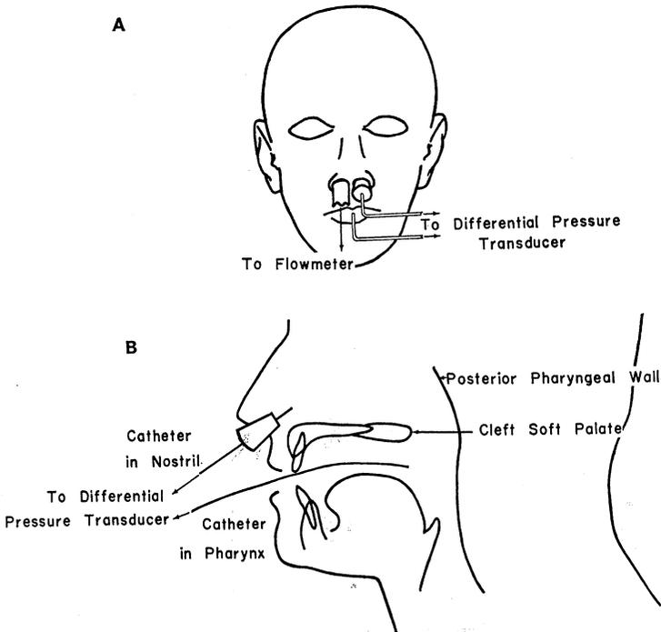
FIGURE 2. The pressure drop across the velopharyngeal orifice is measured by catheters placed in the oropharynx and nasal cavity and attached to a differential pressure transducer. Nasal airflow is measured by a heated pneumotachograph attached to the right nostril.
