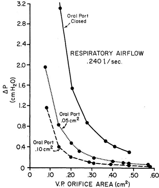
FIGURE 8. The effect of oral port opening on pressure-area relationships. Opening the oral port slightly for simulated fricatives significantly decreases orifice pressure unless airflow rate is increased. The difference in pressure is greatest when velopharyngeal orifice size is small.
