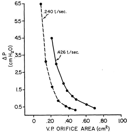
FIGURE 5. The effect of airflow rate on the relationship between orifice pressure and area. As airflow rate increases the curve shifts to the right.
