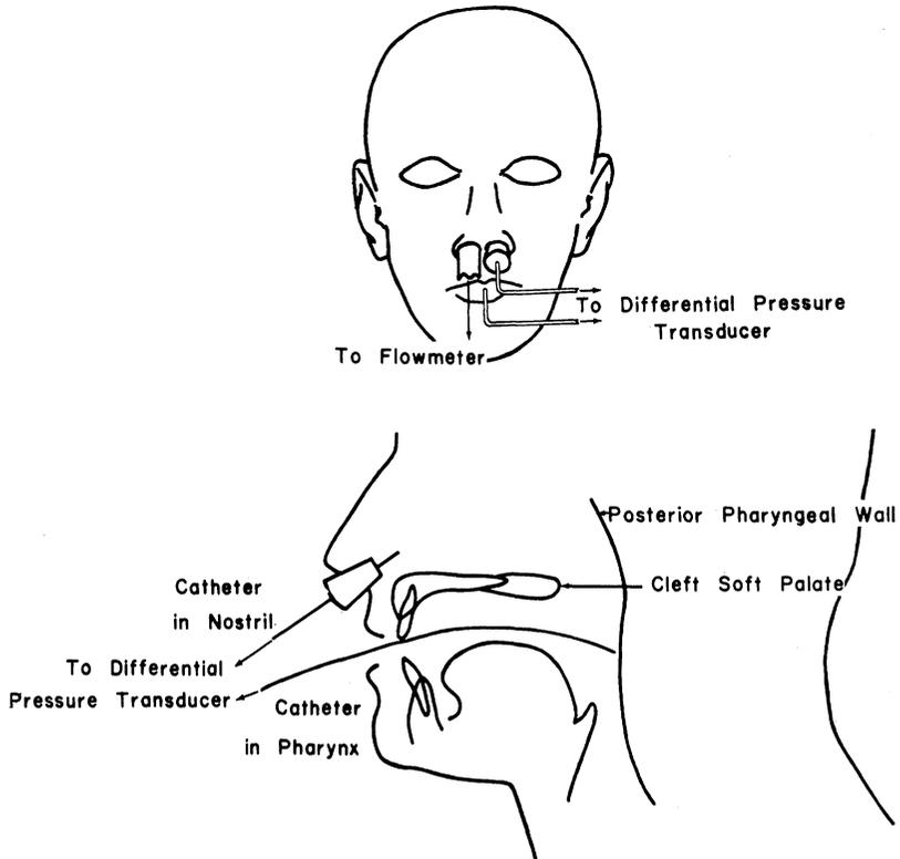
FIGURE 2. Technique for recording orifice pressure drop and nasal airflow for estimation of velopharyngeal orifice size.
