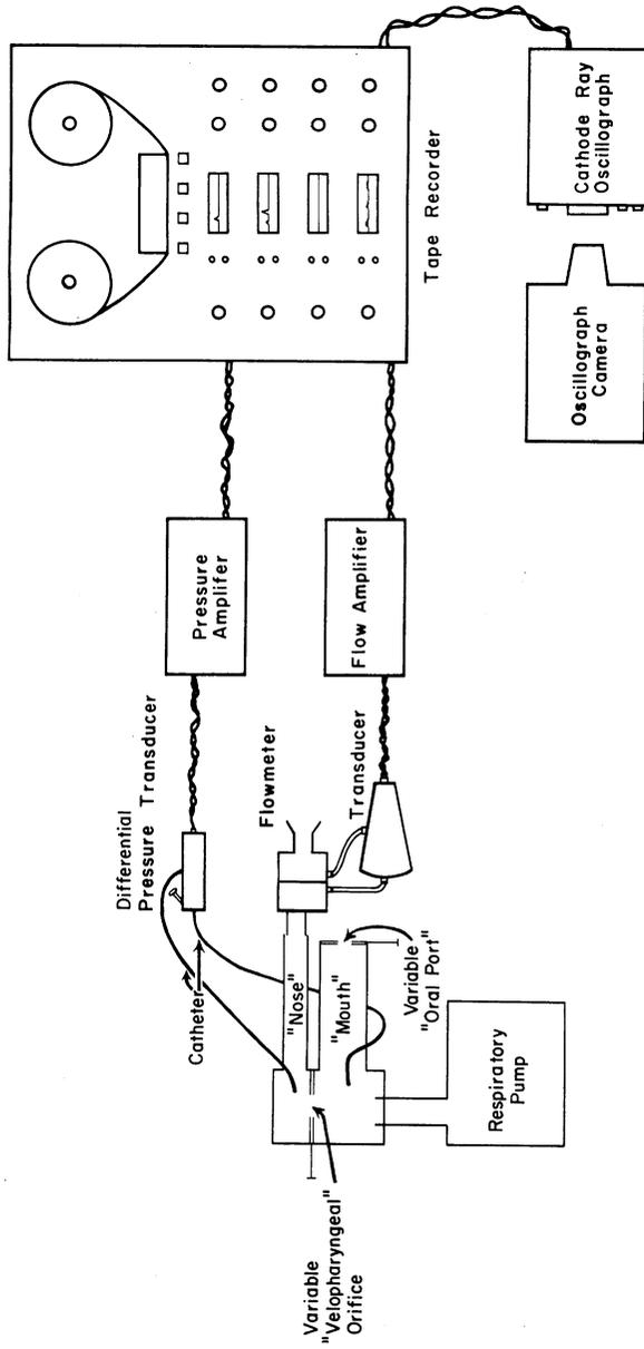
FIGURE 3. Apparatus used to record pressure-flow relationships during simulated speech.
