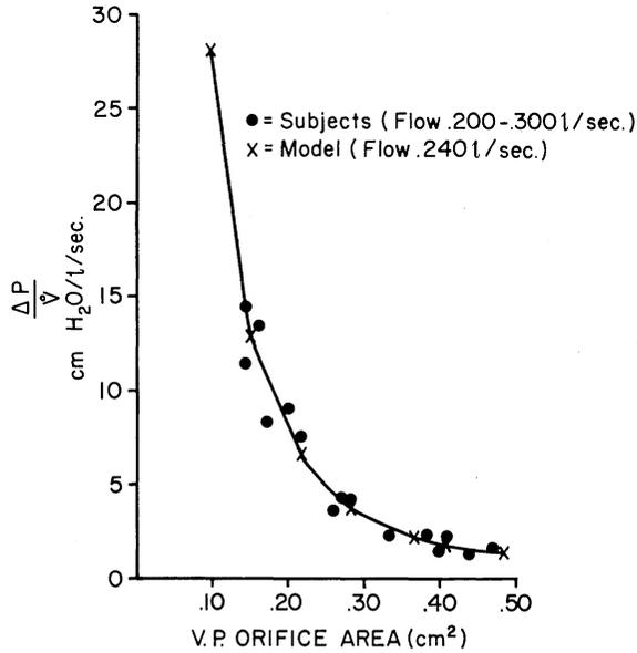
FIGURE 7. The relationship between sphincter resistance to nasal airflow and orifice size. The data presented for both subjects and the model indicate that sphincter resistance impedes nasal airflow significantly when orifice size is below approximately .20 cm<sup>2</sup>.
