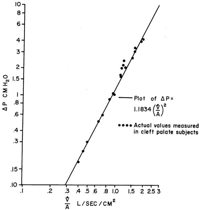
FIGURE 6. A log-log plot of the equation relating orifice pressure drop to rate of nasal airflow and orifice size. Data also presented from the subjects illustrate the closeness of fit.
