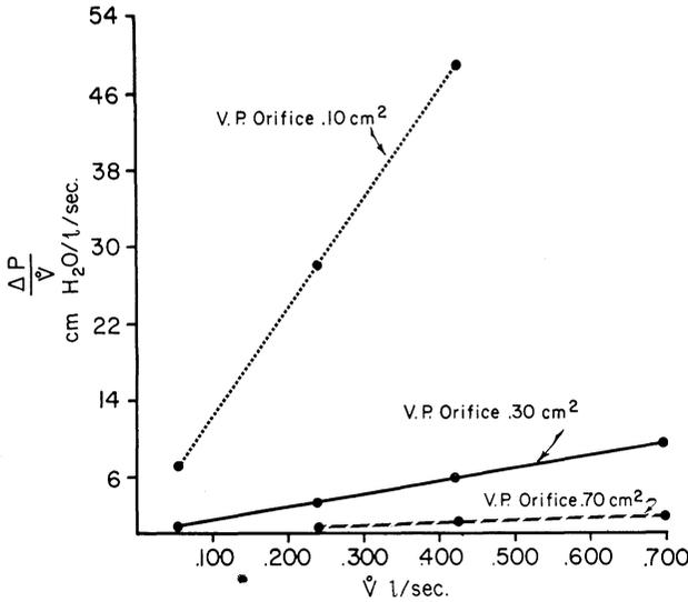
FIGURE 10. The relationship between orifice resistance, respiratory rate, and orifice size. Resistance increases linearly with increasing respiratory airflow rate.
